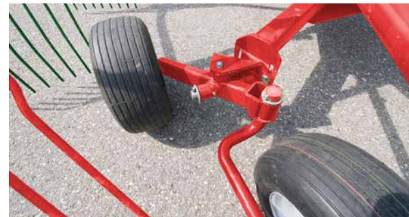
Optional tandem axle for additional stability specially on hillside.
