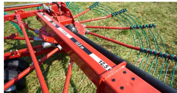
Hydraulic adjustment of working and swath width.
