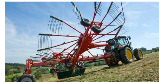
The two rotors are hydraulically lifted on headlands, and ensure outstanding ground clearance in headland position.
