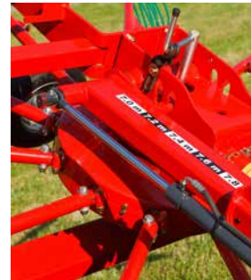
9476 C - Hydraulic 7.0-7.8m working width.
