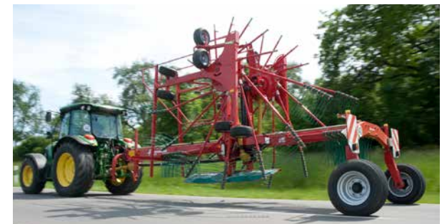
To reach a transport height below 4.00m, the tine arms are removed and safely placed on the carrier frame.
