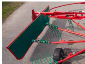
Automatic fold-able swath board with parking stand.
