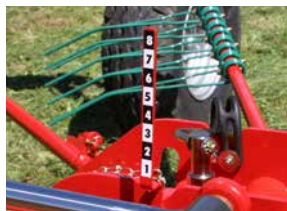
Hydraulic height adjustment of the rotors to suit length of the stubble or varying ground conditions.
