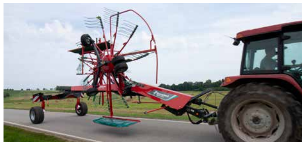
Transport height below 4m.
